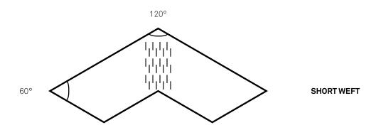
The dotted lines shows the direction of the weft yarn. The weft, is the thinner yarn, which is drawn through the warp, the thicker yarn. Depending on the direction of the weft, a different effect can be seen.
