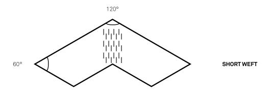
The dotted lines shows the direction of the weft yarn. The weft, is the thinner yarn, which is drawn through the warp, the thicker yarn. Depending on the direction of the weft, a different effect can be seen.
