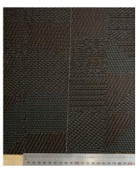
**GEOMETRIC 1.** Overlap 2 sheets of flooring so the pattern repeat of two side-by-side squares is 15 cm. Cut so one square is about 7,5 cm.
