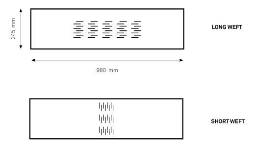
The dotted lines shows the direction of the weft yarn. The weft, is the thinner yarn, which is drawn through the warp, the thicker yarn. Depending on the direction of the weft, a different effect can be seen.
